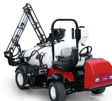
TORO MULTIPRO 1750-G ARBETSBREDD ..... 560CM TANKKAPACITET ..... 662LITER SPRUTTRUCK, ULTRASONIC BOOM, GEOLINK
